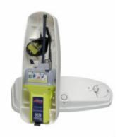
An EPIRB is a radio beacon that transmits your location in case of an emergency and usually deploy themselves when found in the water for instance when a vessel is sinking. They need to be registered for emergency services to be able to know what type of vessel is in trouble etc. They can also be attached to a life raft/vest to be able to find survivors after an emergency.
