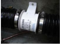
Gasoline fumes are highly explosive and can cause serious injuries or death when ignited. If fuel lines and/or filters are running through compartments that also house automatic pumps or other equipment some form of ventilation is needed.
