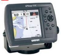
A Global Positioning System device allows a captain/crew to always know where they are. This information greatly reduces time needed to find vessels in distress by Search and Rescue operations.
